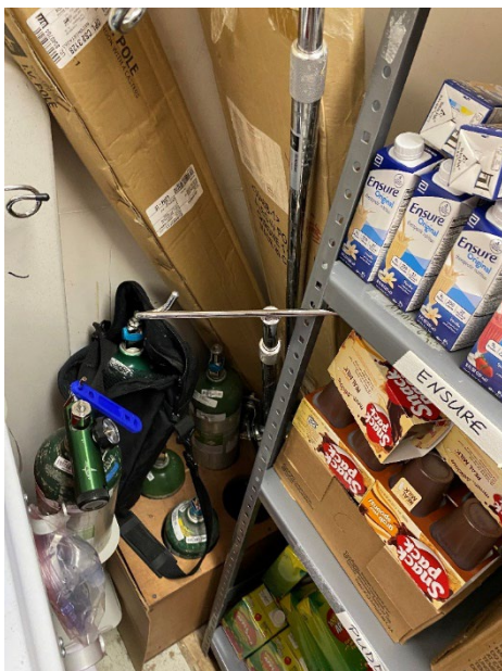
Photograph 8: Improperly stored oxygen tanks.
