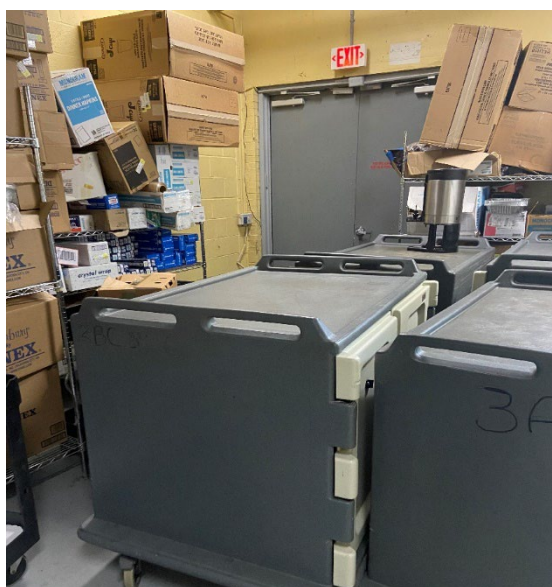
Photograph 3 (left): Pathway to exit blocked by storage. Photograph 4 (right): Smoke barrier self-closing door not closing properly (broken mechanism).
