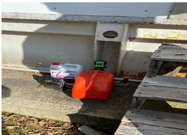
Photograph 7: Hazardous chemical (i.e., gas) not stored in a safe manner (i.e., in an approved safety storage cabinet).
