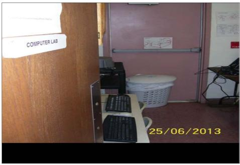
Photograph 1: A fire exit blocked by a garbage can.
